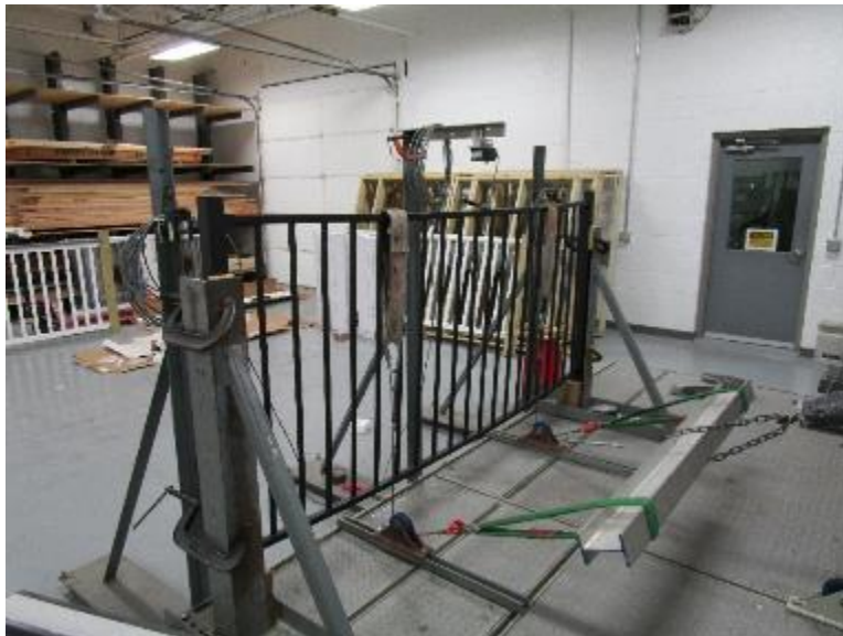
Photo No. 4 Vertical Uniform Load on Top Rail
