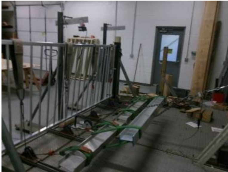
Photo No. 4 Vertical Uniform Load Test on Top Rail
