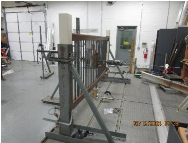
Photo No. 1 In-Fill Load Test at Center of Three Pickets
