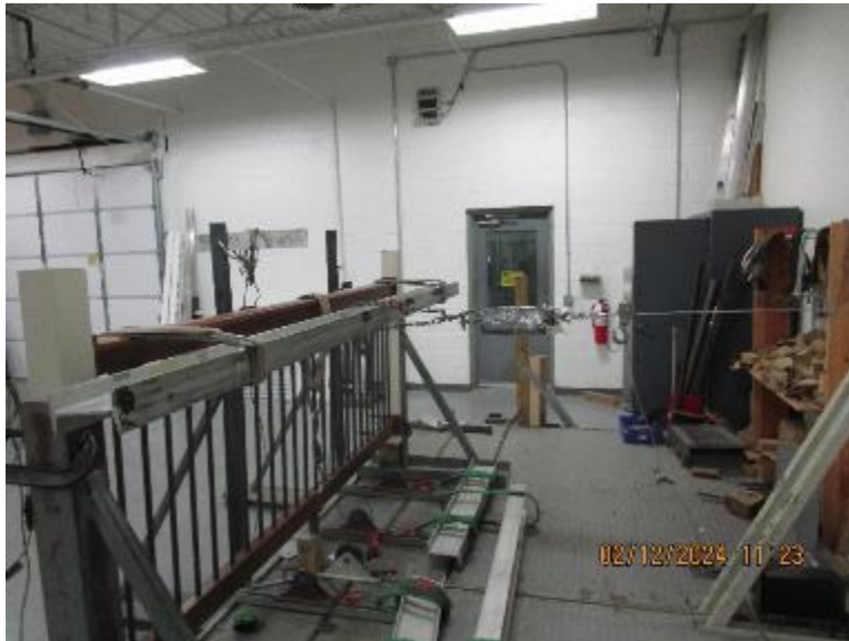
Photo No. 6 Horizontal Concentrated Load Test at Ends of Top Rail (Brackets)
