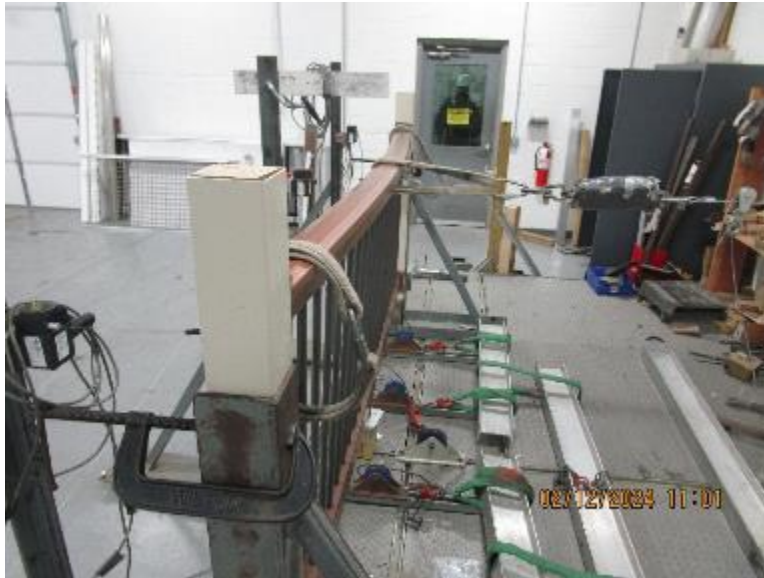
Photo No. 5 Horizontal Concentrated Load Test at Mid-Span of Top Rail
