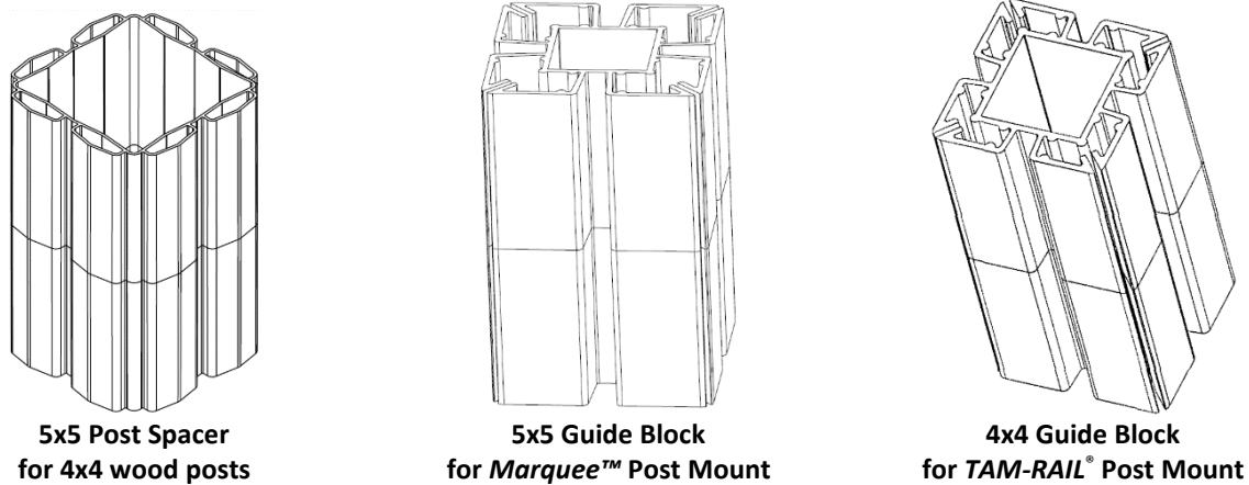
FIGURE 8 – POST SPACERS & GUIDE BLOCKS
